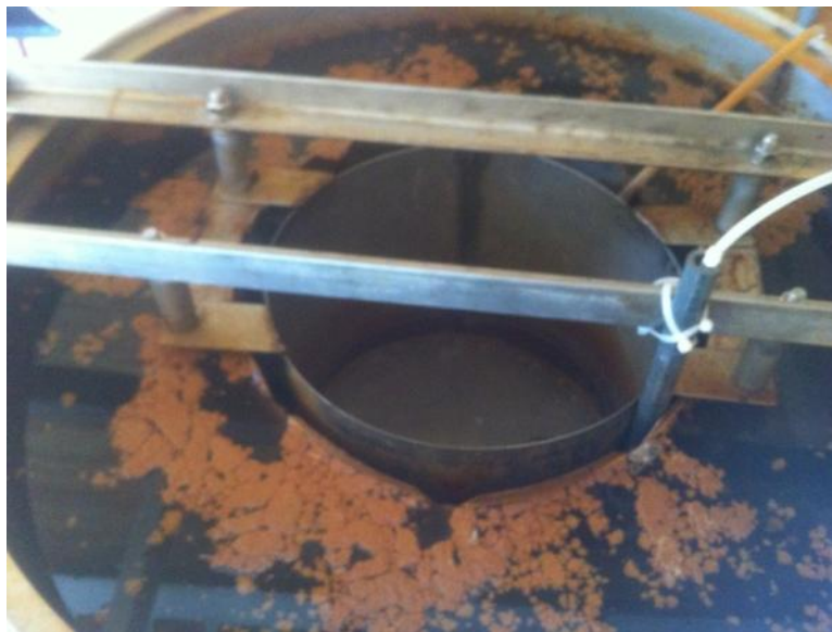
Figure 3. Top interior of redesigned Site A pilot bead filter
